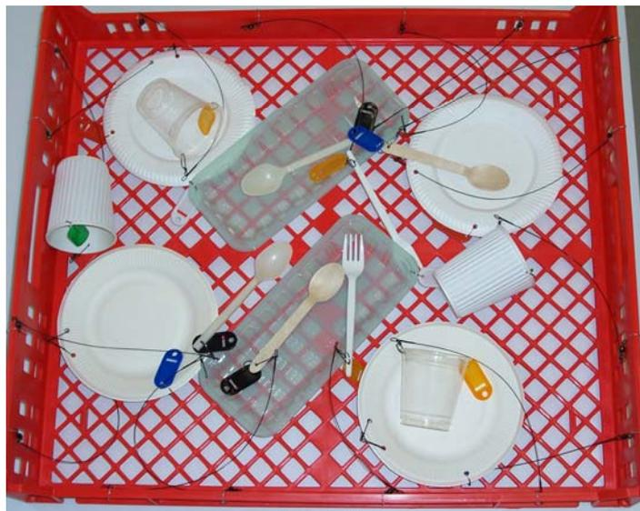
Figure 1: A typical sample tray prior to burial in a compost pile
